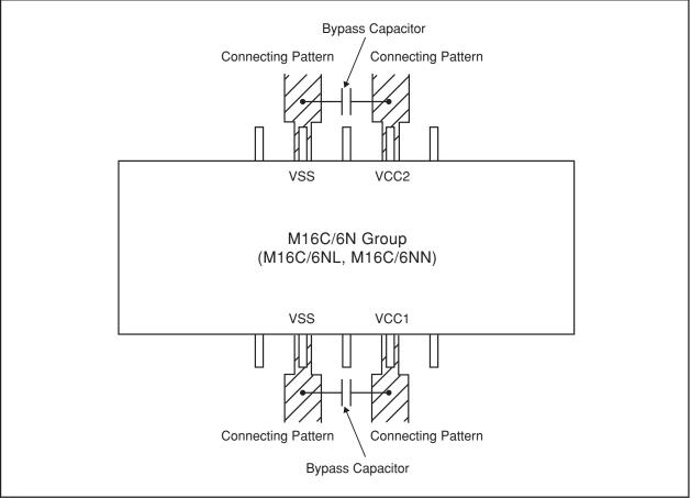
Figure 22.11 Bypass Capacitor Connection
